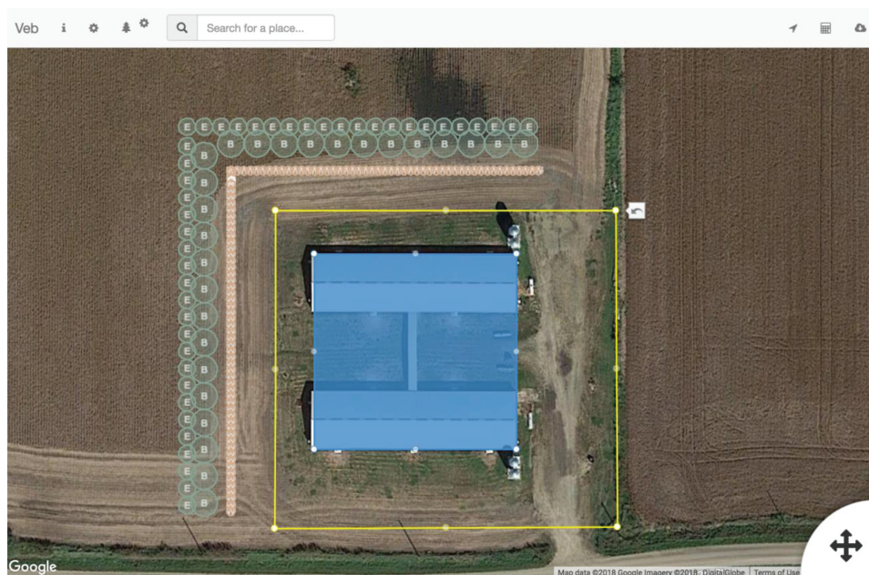
Figure 4. Design displaying a simple three-row VEB located around the west and north sides of a three-building, naturally ventilated animal building; tree species were selected based on soils include Eastern red cedar ( Juniperus virginiana ) in the outside row, hybrid willow ( Salix spp. ) in the middle row and Ninebark ( Physocarpus opulifolius ) on the inside.
